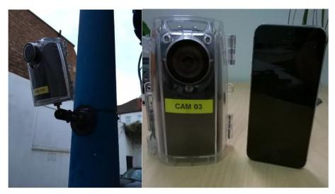
Our cameras collect wide angle, high-definition views to enable accurate identification and classification of movements. A typical view captured by our cameras is shown below. We will use high-capacity batteries and recording media within our cameras to help ensure continuous, uninterrupted recording of images throughout the survey period, and synchronise all cameras together to ensure ease of analysis at a later stage.
